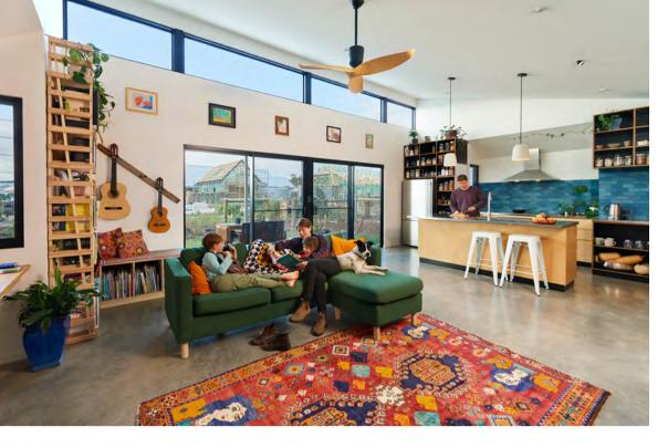
Clerestory windows flood the living space with natural light, and a concrete slab floor functions as thermal mass. The home's design meets Livable Housing Australia's Silver Level guidelines for accessibilty, including step-free access, generous circulation spaces and wide doorways.
